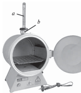
22-rasm. Termostat (quritgich shkaf): a—termometr; b—ventilatsiya teshiklari.
