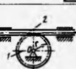
19.2.5. Radiuslari  $r_1=0,15\text{m}$  va  $r_2=0,3\text{m}$ , aylanish o'qiga nisbatan inersiya momentlari  $J_1=0,02\text{kg m}^2$  va  $J_2=0,04\text{kg m}^2$  bo'lgan tishli g'ildirakli mexanizmga momenti  $M_1=0,15\text{N}\cdot\text{m}$  ga teng bo'lgan juft kuch ta'sir etsa, 1 g'ildirakning burchak tezlanishini toping. (5)
