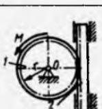
19.2.7. Radiuslari  $r_1=0,05\text{m}$  va  $r_2=0,1\text{m}$ ; aylanish o'qlariga nisbatan inersiya momentlari  $J_1=0,01\text{kg m}^2$  va  $J_2=0,02\text{kg m}^2$  bo'lgan shkivlar momenti  $M=0,15\text{N}\cdot\text{m}$  li juft kuch ta'sirida harakatga kelsa, 1 shkivning burchak tezlanishini aniqlang. (10)
