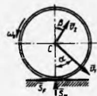
**22.4.5.** Massasi  $m=0,6\text{kg}$  bo'lgan disk  $\omega_0=2\text{rad/s}$  burchak tezlik bilan aylanib, massa markazi  $v_0=1,8\text{m/s}$  tezlikka ega holda vertikal devorga  $\alpha=45^\circ$  burchak ostida uriladi. Agar normal impulsning tiklash koeffitsiyenti  $k=0,55$  bo'lsa, normal impuls  $S_N$  ning qiymatini hisoblang. (1,18)
