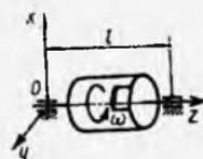
**17.4.21.** Rotor juft kuch momenti  $\bar{M}$  ta'sirida  $\omega=10\text{rad/s}$  burchak tezlik va  $\varepsilon=60\text{rad/s}^2$  burchak tezlanish bilan  $Oz$  o'qi atrofida aylanadi. Agar rotoring markazdan qochma inersiya momentlari  $J_{xz}=0$ ,  $J_{yz}=5 \cdot 10^{-3} \text{ kg}\cdot\text{m}^2$  bo'lib, podshipniklar  $\ell=0,25\text{m}$  masofada bo'lsa,  $O$  podshipnikdagi dinamik reaksiya kuchini aniqlang. (2,33)
