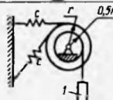
**19.3.24.** Massalari  $m_1=1\text{kg}$  va  $m_2=2\text{kg}$  bo'lgan ikki jism shkv vositasida bikirligi  $c=100\text{N/m}$  li prujinaga osilgan holda tebransa, 1 jismning erkin vertikal tebranishlarining chastotasini aniqlang. (6,67)
