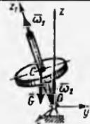
**16.3.3.** Inersiya momenti  $J_{z1}=0,001\text{kg}\cdot\text{m}^2$  bo'lgan pirildoq  $\omega_1=100\text{rad/s}$  va  $\omega_2=1,4\text{ rad/s}$  burchak tezliklari bilan muntazam pretsessiyada bo'lib,  $\bar{\omega}_1$  va  $\bar{\omega}_2$  larning orasidagi burchak  $\theta=5^\circ$  bo'lsa, uning og'irlilik kuchi  $\bar{G}$  ning  $O$  nuqtaga nisbatan momentini hisoblang. ( $1,22 \cdot 10^{-2}$ )
