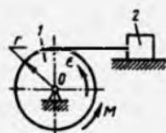
17.3.17. Vibrator ikki sinxon aylanuvchi pnevmoturbinalardan iborat bo'lib, ularning valiga  $r=10\text{sm}$  masofada  $m=0,5\text{kg}$  massalar o'rmatilgan. Agar trubinalar  $n=1000\text{ayl/min}$  chastotasi bilan aylansa, vibrator asosiga ko'rsatilayotgan eng katta dinamik zo'riqishni toping (kN). (1,10)
