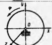
**16.1.4.** Vertikal o'q atrofida aylanuvchi sterjen  $\varphi=3t-t^3$  tenglama asosida aylansa, uning inersiya momentini  $J_z=1/6\text{kg}\cdot\text{m}^2$  deb, sterjenga ta'sir etuvchi tashqi kuchlarning bosh momentini aniqlang. (1)
