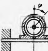
**17.3.23.** Massasi  $m=5\text{kg}$ , inersiya radiusi  $\rho=0,07\text{m}$ , radiusi  $r=0,1\text{m}$  bo'lgan tishli g'ildirak  $M=10\text{N}\cdot\text{m}$  juft kuch momenti ta'sirida  $\varepsilon=200\text{rad/s}^2$  burchak tezlik bilan aylansa, 2 tishli g'ildirakka  $L$  tishlashish chizig'ida ta'sir qiluvchi kuchning modulini toping. (54,3)
