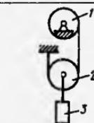
**19.2.13.** Radiuslari teng  $r=0,2\text{m}$ , massalari bir xil  $m_1=m_2=1\text{kg}$ , markaziy o'qqa nisbatan inersiya momentlari  $J_1=J_2=0,02\text{kg}\cdot\text{m}^2$  bo'lgan g'ildiraklar o'zgarmas momentli  $M=0,2\text{N}\cdot\text{m}$  juft kuch ta'sirida harakat qilsa, 1 g'ildirakning burchak tezlanishini aniqlang. (2,5)
