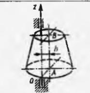
**16.1.21.** Devorga qistirib mahkamlangan  $OA$  konsol to'sinning uchiga rotor o'rnatilgan bo'lib, u tiklovchi moment  $M_z=-\pi^2\varphi$  ta'sirida  $\varphi=3\sin(\pi/4)t$  qonun bilan burilma tebranishda bo'lsa, rotorning  $Az$  o'qiga nisbatan inersiya momentini hisoblang. (16)
