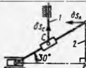
18.2.9. Press mexanizmi shatunining  $A$  va  $B$  nuqtalari mumkin bo'lgan ko'chishlari  $\delta s_A$  va  $\delta s_B$  ning nisbatini aniqlang. Bunda  $OA=AB$  va  $\alpha=30^\circ$  deb olinsin. (1,73)
