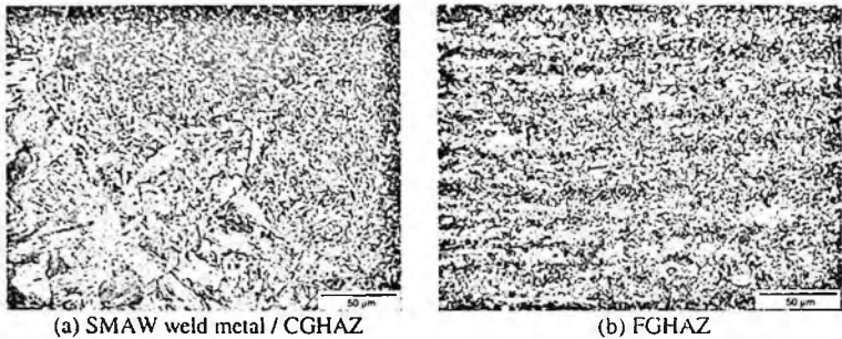
Fig. 1. Microstructures in girth weld of X80 pipeline.
