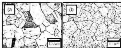
Fig. 1. Microstructures of (a) Inconel 600 and (b) Inconel 690.
