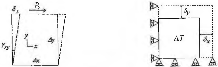
Fig. 3. Unit cell: (a) under the pure shear; (b) under the uniform thermal expansion.
