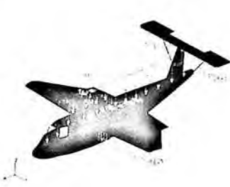
Figure 7. FE model for structural analysis
