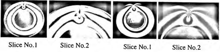
Figure 2. Isochromatic fringe pattern (Type C) Figure 3. Isochromatic fringe pattern
