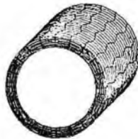
Fig. 1. Torsional vibration mode in a pipe.
