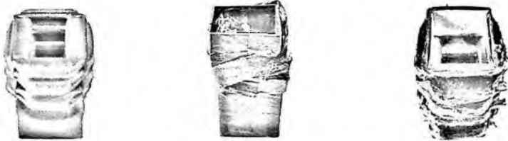
(a) Aluminum square member (b) CFRP square member (c) Aluminum/CFRP square member Figure 2. Collapse modes of square member
