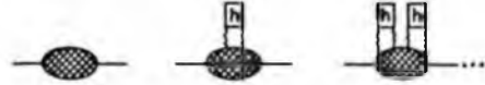
FIG. 8. Grouping of the electron proper self-energy into contributions involving no factors h , exactly one factor h , exactly two factors h , etc. The shaded blobs are calculated with all internal photons described by free propagators coupling with the asymptotic coupling strength \alpha_0 .
