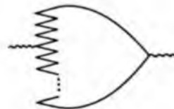
FIG. 10. Ordering in which a single-fermion vacuum-polarization loop diagram describes the creation of an infinite number of pairs from the vacuum. (We have not drawn in any of the internal photons.)
