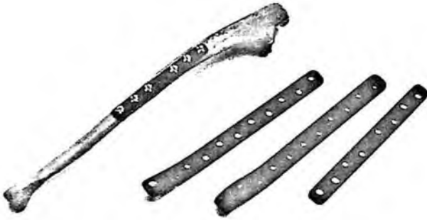
Fig. 1.5 Carbon fiber reinforced epoxy composite bone plates (Evans and Gregson, Bio-materials , Vol. 19, No. 15, pp. 1329–1342, 1998).
