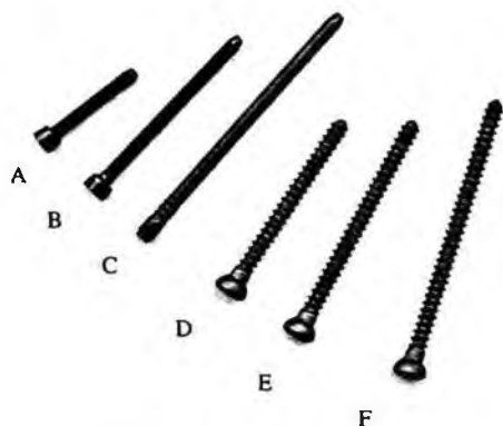
Fig. 1.3 Endless carbon fiber reinforced PEEK matrix medical screws made by Composite Flow Molding, carbon fiber volume content 62% (by courtesy of Icotec AG, Switzerland) [R. Tognini, Ph.D. Thesis, ETH Zurich, 2001].
