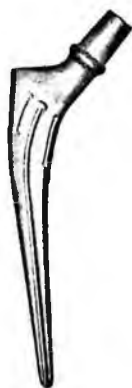
Fig. 1.4 Hip endoprosthesis stem, injection molded, chopped long fiber reinforced PEEK, fiber volume content 50% [M. Semadeni, Ph.D. Thesis, ETH Zurich, 1999].
