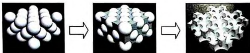
Figure 1. General steps in the preparation of 3DOM solids by colloidal crystal templating.
