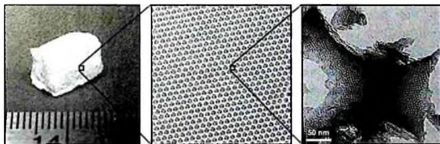
Figure 5. Monolithic silica with hierarchical porosity. The photograph on the left shows the monolith with millimeter edge lengths. The macropore arrays are apparent in the SEM image in the middle. The TEM image on the right shows cubic mesopores in the silica walls that surround macropores.
