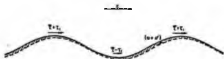
FIG. 1. The boundary layer at the free surface induced by a tangential stress in phase with the surface elevation. The boundary layer is thickest on the rear slope of the wave.
