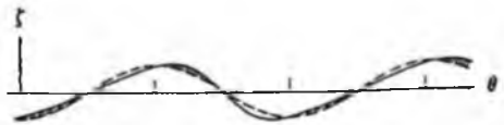
FIG. 4. Schematic diagram showing how skewness of individual waves can arise from a second harmonic.
