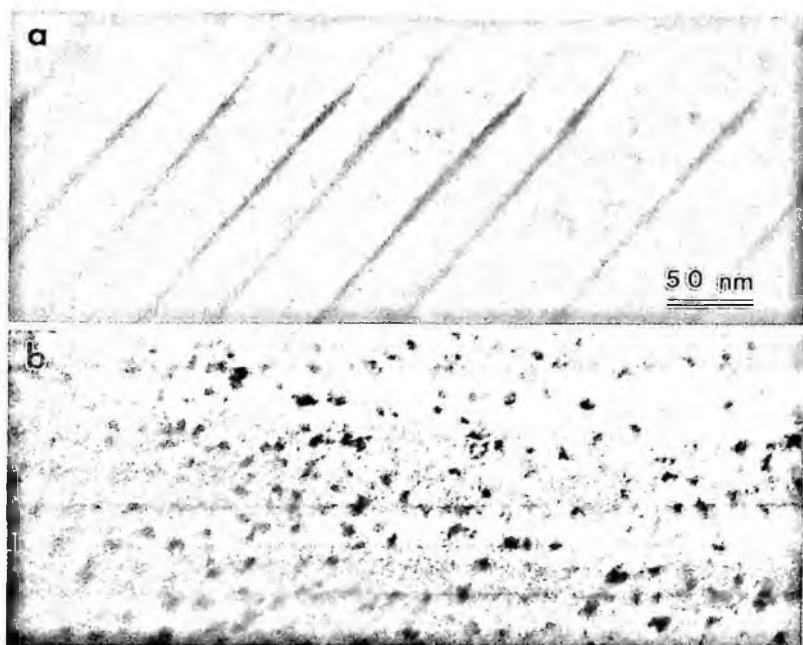
Figure 13.4 The degree of the radiation damage seen in TEM caused by Cu ions varies with the electron beam near the [001] axis of two different regions of a sample of \text{YBa}_2\text{Cu}_3\text{O}_{7-\delta} ( 0 < \delta < 0.1 ). Note the defects do not exhibit the same type of strain contrast shown by “regular” columns, as in Fig.13.2. In some areas, even the weak strain contrast seen in (b) cannot be observed. [The approximately linear features seen in (a) and (b) are twin boundaries.]
