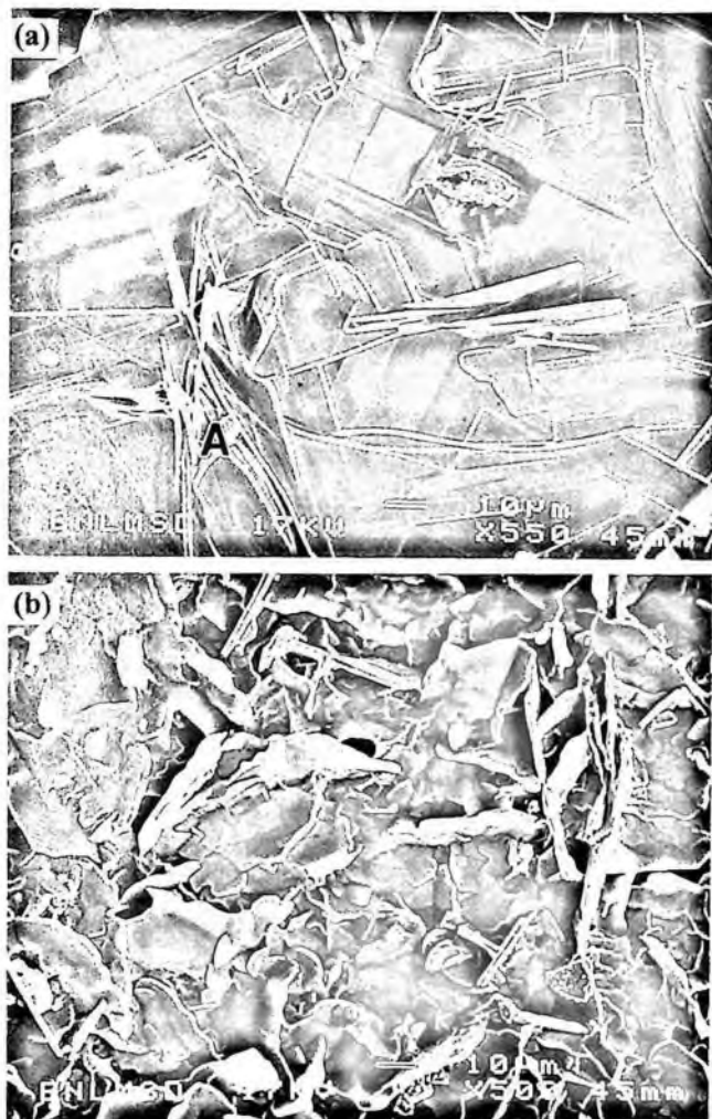
Figure 12.18 Scanning electron micrographs of (a) Bi-2212/Ag, and (b) Bi-2223/Ag tapes viewed along tape-normal incidence after Ag removal.
