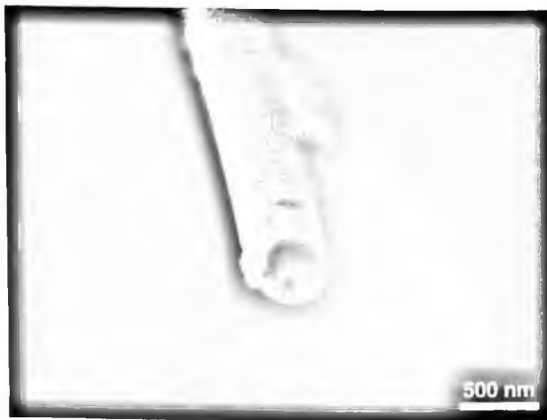
Figure 5. SEM image of the circular cross section of a 480-nm thick nanowire.
