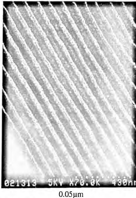
Figure 45. The replicated patterns with a size of 0.05 μm replicated by AT&T.
