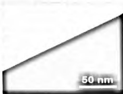
Figure 11. TEM examination of the sidewall of a 210-nm thick phosphate glass nanowire. (Adapted from Ref. [16].)
