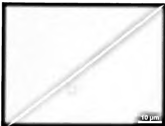
Figure 12. Optical microscope image of a 60-nm thick silica nanowire supported by a silicon wafer. The image is taken in dark-field reflection mode.
