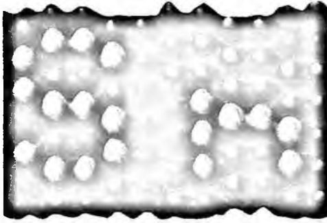
Figure 14. AFM image ( 7.7 \times 7.7 \text{ nm}^2 image size) of atom inlaid letter “Sn” by rearranging Sn atoms on Ge(111)-c( 2 \times 8 ) surface at room temperature with cantilever oscillation amplitude of 15.7 nm, using Si cantilever of 29.5 N/m spring constant, setting frequency shift value of -4.6 \text{ Hz} with respect to first-mechanical resonant frequency of 160 kHz (courtesy of Dr. Oscar Custance of Osaka University, Japan).
