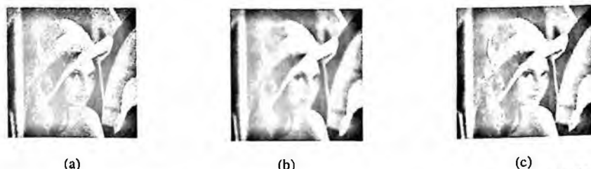
Fig. 1. (a) Lena image corrupted with Gaussian noise of variance \sigma_n^2 = 924 ( PSNR = 20dB ). (b) PM anisotropic diffused image after 10 iterations with \sigma_n^2 = 153.3 and PSNR = 26.3dB (c) Output of the ALSAF after 10 iterations with \sigma_n^2 = 137.6 and PSNR = 26.8dB .
