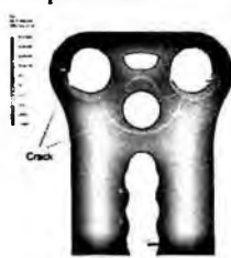
Fig. 7. The Position of the Crack
