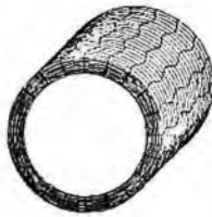
Fig. 1. Torsional vibration mode in a pipe.
