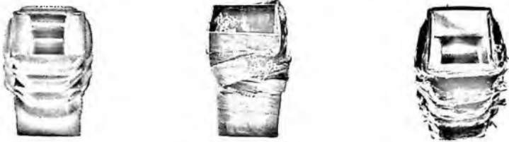
(a) Aluminum square member (b) CFRP square member (c) Aluminum/CFRP square member Figure 2. Collapse modes of square member
