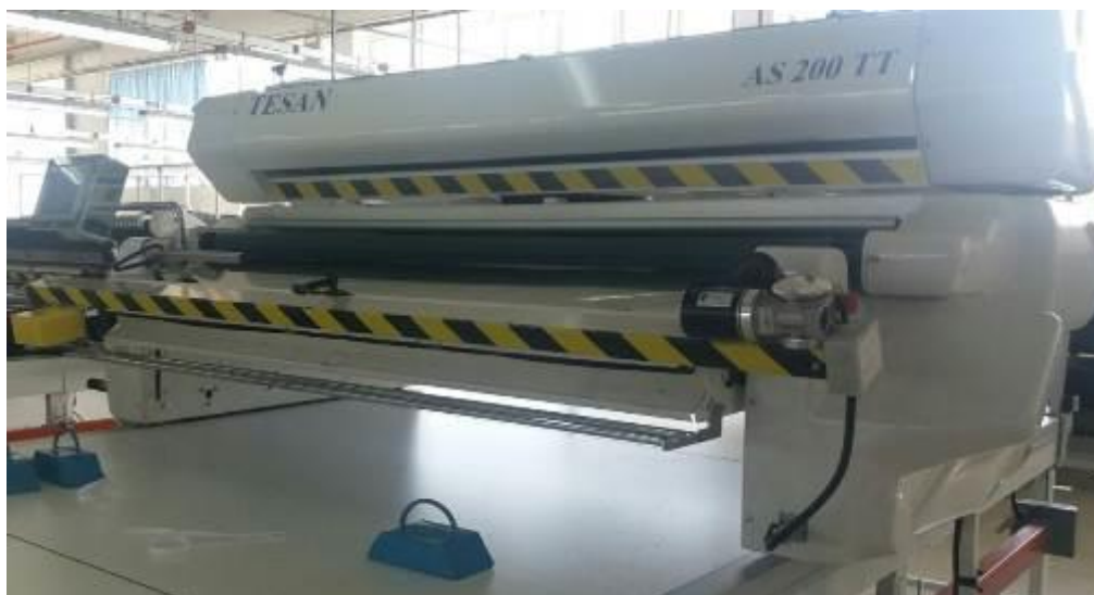
10-rasm. "TESAN AS 200 TT" markali gazlamalarni to`shash jihozi
