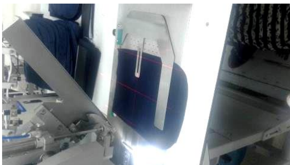
62-rasm. Mag`izli qirqma cho`ntakni tikish uchun lazer nuri tushirish jarayoni
