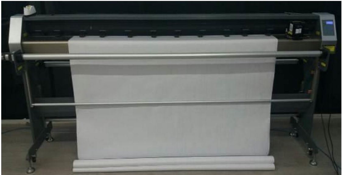
2-rasm. Andozlarni M 1:1da chop etadigan PLOTTER qurilmasi
