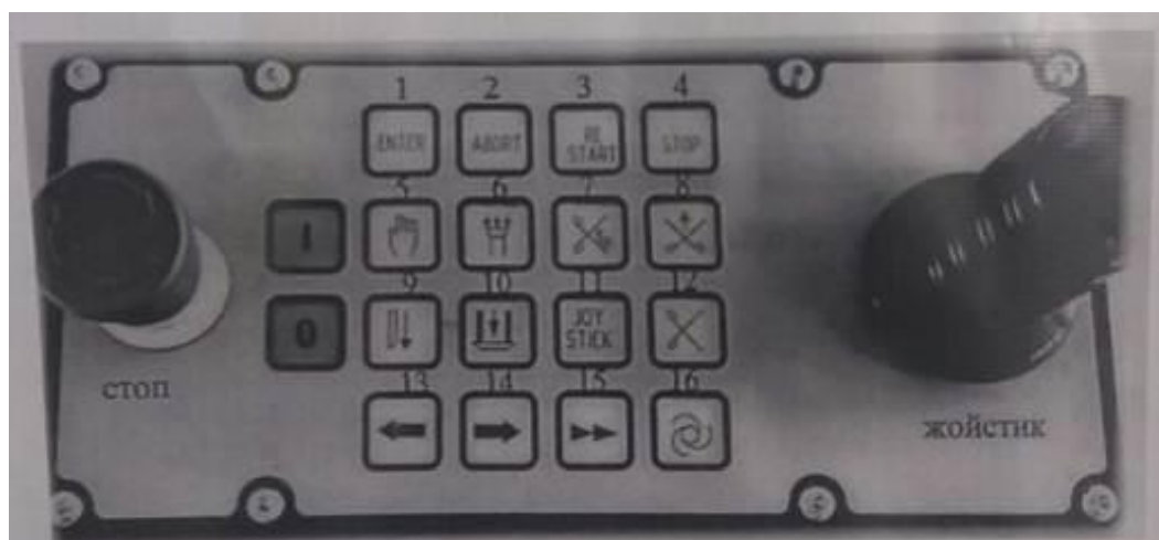
14-rasm. BULMER bichuv dastgohini ishga tushirish sxemasi
