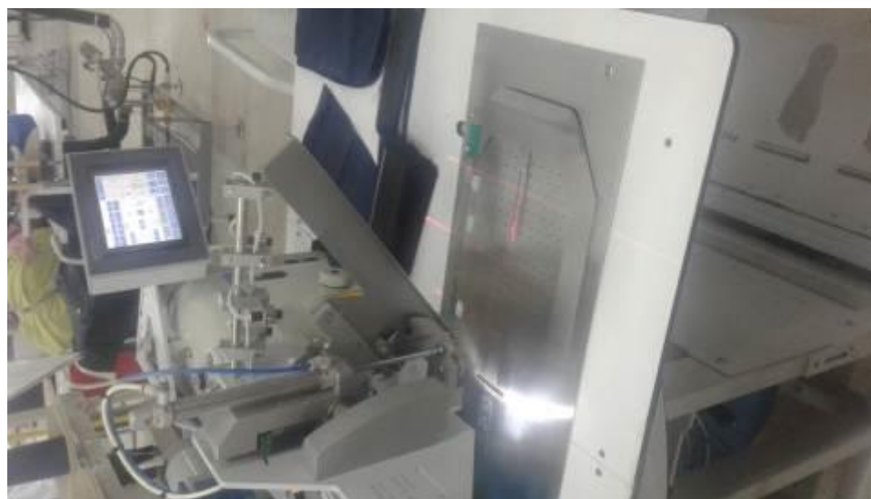
62-rasm. Mag`izli qirqma cho`ntakni tikish uchun lazer nuri tushirish jarayoni
