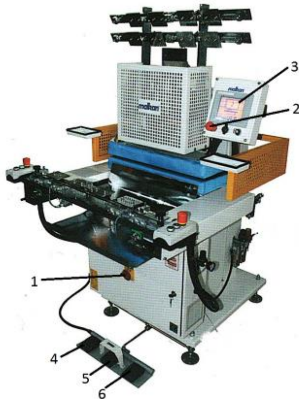
36-rasm. Cho`ntak klaponini pnevmatik press qilish dastgohi Shimming old bukloviga shakl beruvchi pressidan foydalanish
