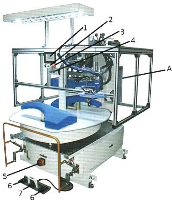
42-rasm. "Karusel" tizimida ishlovchi kostyumning yeng orqa chokini presslovchi dastgoh
