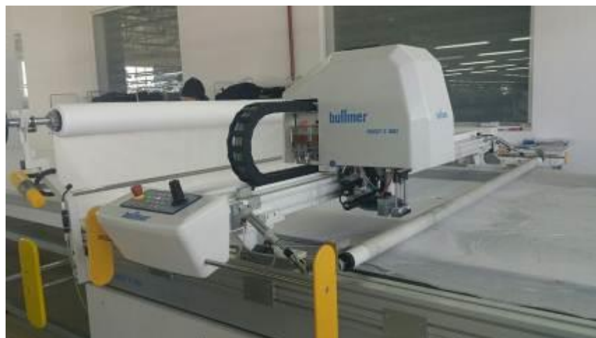
15-rasm. Maxsus lazer va pichoqli BULMER PROCUT D 8003 markali jihozining ko`rinishi
