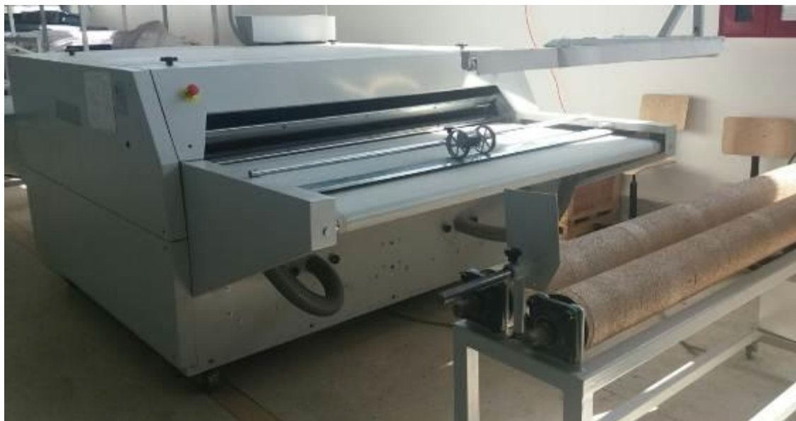
9-rasm. Gazlama sifatini tekshiradigan va nuqsonini aniqlaydigan K 1600 MM markali maxsus dastgoh.
