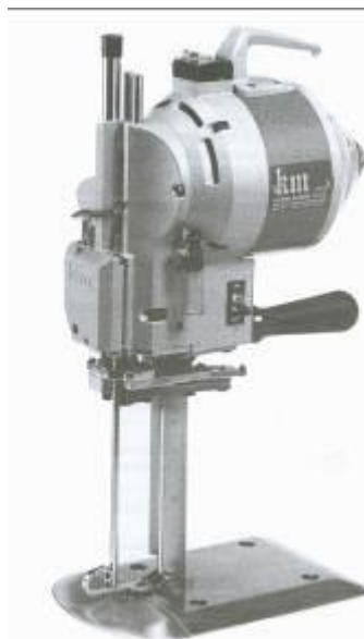
21-rasm. KS-AUV tik pichoqli ko`chma bichish mashinasi
