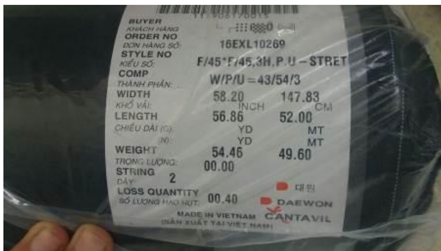
7-rasm. Plyonka qoplamadagi gazlama ruloni va uning pasporti
