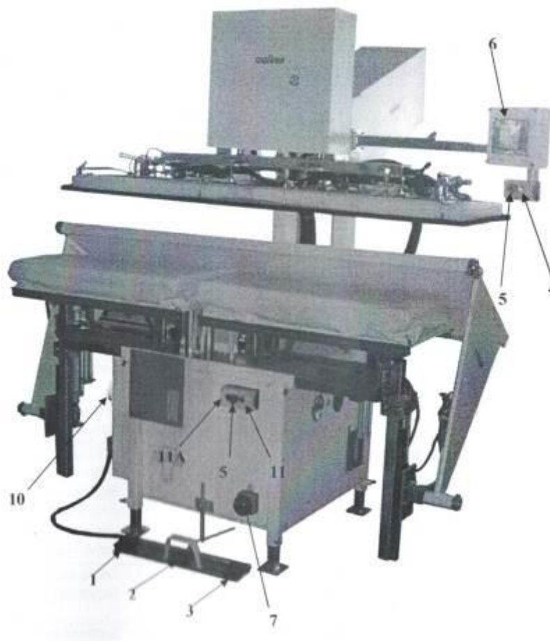
45-rasm. Shimning dazmol yo`lini ochish pressi
