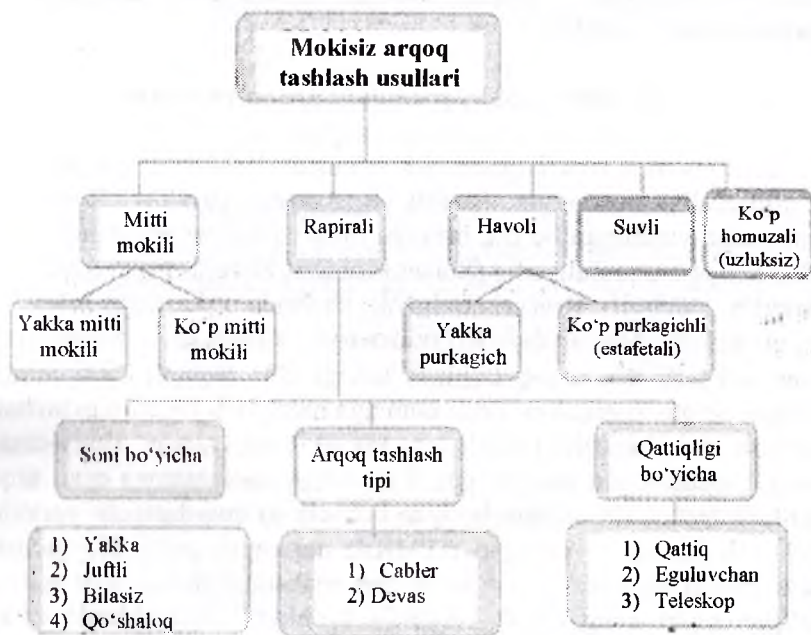
3.8-rasm. Mokisiz arqoq tashlash usullari
