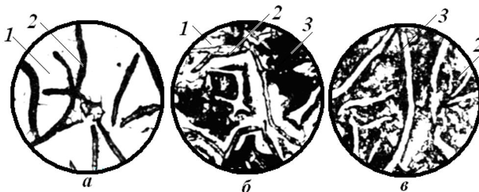
5.23 – rasm. Kulrang cho'yanni mikro tuzilmasi: a – ferritli, b – ferrit – perlitli, v – perlitli, 1 – ferrit; 2 – plastinkali grafit; 3 – perlit.
