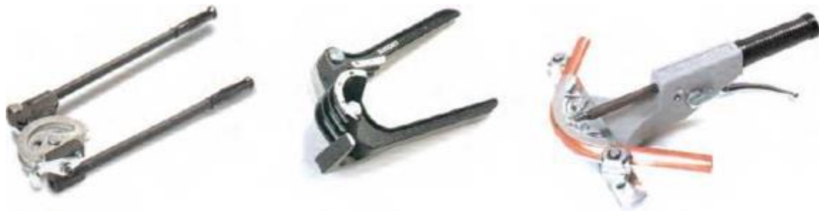
Figure 3.12. Yexamples of ‘and ‘eld bending machines (Reproduced wit’ permission of Ridgid Tools) 1
