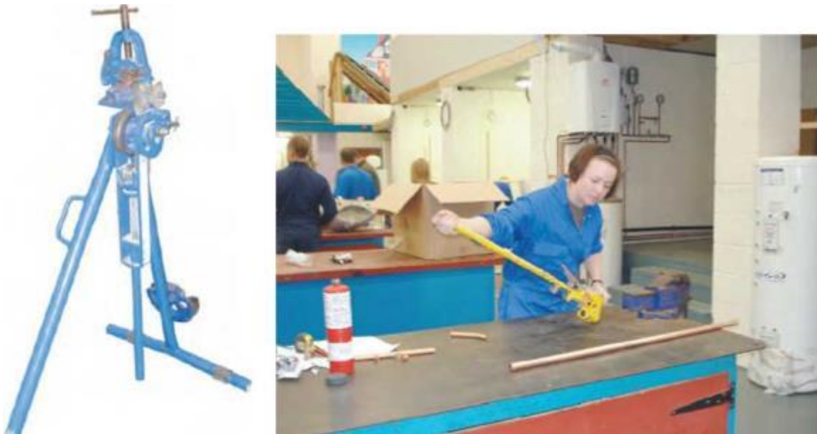
Figure 3.12. Yexamples of ‘and ‘eld bending machines (Reproduced wit’ permission of Ridgid Tools) 1
