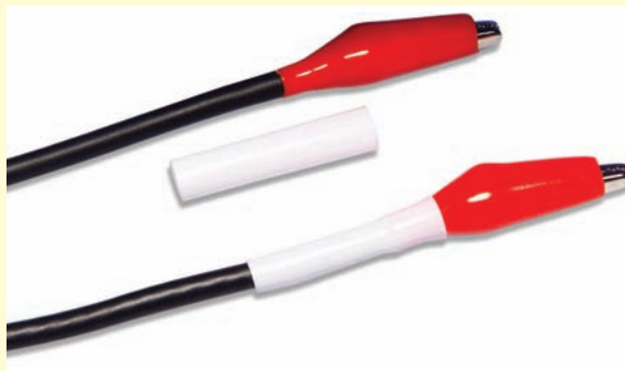
Photograph showing (from top to bottom) an electrical connection, a piece of as-received polymer shrink-tubing, and the constricted tubing around the junction—application of heat to the tubing caused its diameter to shrink. (Photography by S. Tanner.)
