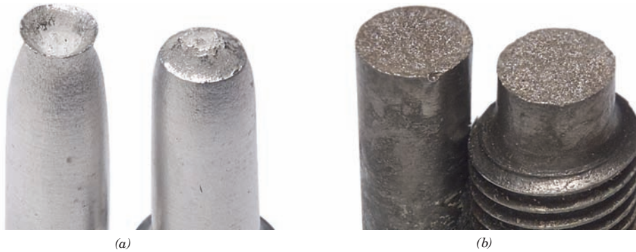
Figure 9.3 (a) Cup-and-cone fracture in aluminum. (b) Brittle fracture in a mild steel.
