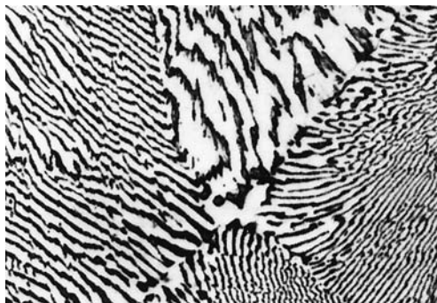
Figure 10.14 Photomicrograph showing the microstructure of a lead–tin alloy of eutectic composition. This microstructure consists of alternating layers of a lead-rich \alpha -phase solid solution (dark layers), and a tin-rich \beta -phase solid solution (light layers). 375 \times . (Reproduced with permission from Metals Handbook , 9th edition, Vol. 9, Metallography and Microstructures , American Society for Metals, Materials Park, OH, 1985.)
