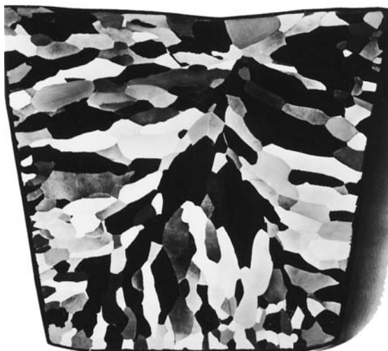
Figure 5.17 High-purity polycrystalline lead ingot in which the individual grains may be discerned. 0.7\times . (Reproduced with permission from Metals Handbook , Vol. 9, 9th edition, Metallography and Microstructures , American Society for Metals, Metals Park, OH, 1985.)
