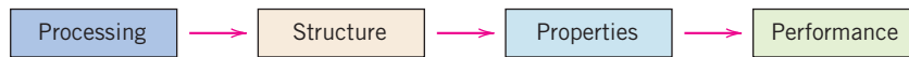
Figure 1.1 The four components of the discipline of materials science and engineering and their interrelationship.
