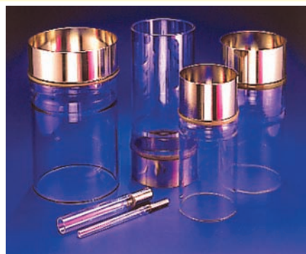
Photograph showing tubular products that have glass-to-metal junctions. The thermal expansion coefficient of the metal alloy (Kovar) is approximately the same as that of the Pyrex glass. Thus, with changes in temperature, the likelihood of the establishment of thermal stresses and fracture at the junction are minimized. [Photograph courtesy of Moores (EVIC) Glassworks, Ltd., Walton-on-Thames, England.]
