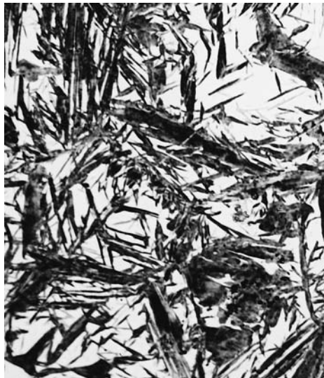
Figure 11.22 Photomicrograph showing the martensitic microstructure. The needle-shaped grains are the martensite phase, and the white regions are austenite that failed to transform during the rapid quench. 1220\times . (Photomicrograph courtesy of United States Steel Corporation.)
