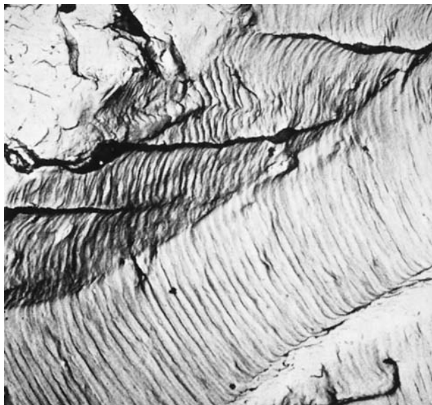
Figure 9.29 Transmission electron fractograph showing fatigue striations in aluminum. Magnification unknown. (From V. J. Colangelo and F. A. Heiser, Analysis of Metallurgical Failures , 2nd edition. Copyright © 1987 by John Wiley & Sons, New York. Reprinted by permission of John Wiley & Sons, Inc.)
