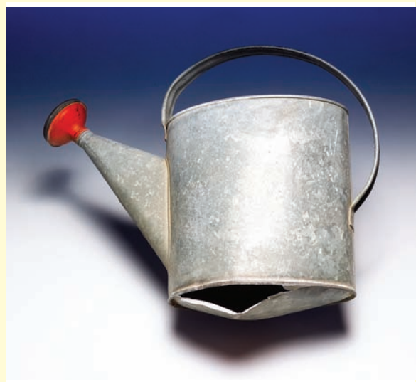
A watering can that ruptured along a side panel-bottom panel seam. Water that was left in the can during a cold late-autumn night expanded as it froze and caused the rupture. (Photography by S. Tanner.)
