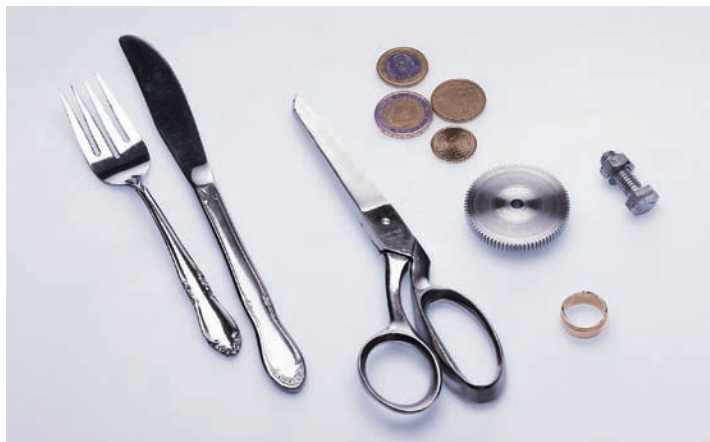
Figure 1.8 Familiar objects that are made of metals and metal alloys (from left to right): silverware (fork and knife), scissors, coins, a gear, a wedding ring, and a nut and bolt. (Photography by S. Tanner.)
