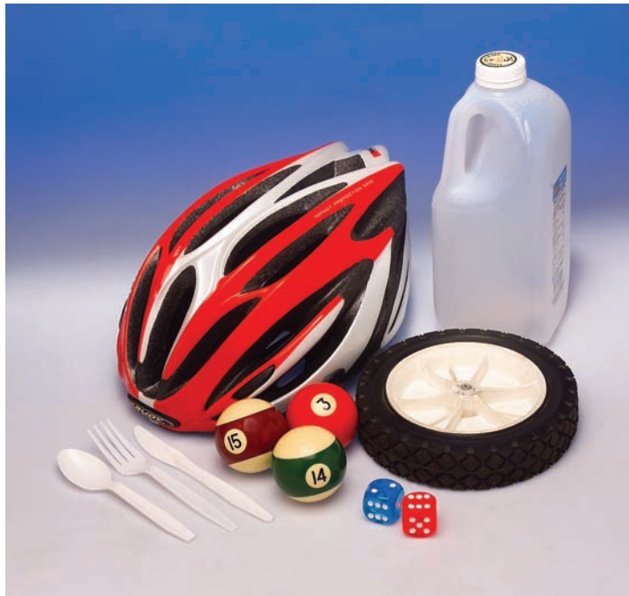
Figure 1.10 Common objects that are made of polymeric materials: plastic tableware (spoon, fork, and knife), billiard balls, a bicycle helmet, two dice, a lawnmower wheel (plastic hub and rubber tire), and a plastic milk carton. (Photography by S. Tanner.)
