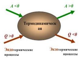
Figure 4 – Sign rule adopted in thermodynamics for heat and work
