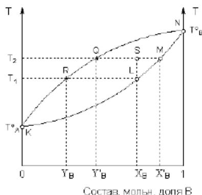
*Rice. 12. Type 1 system state diagram in temperature–composition coordinates ( $p = \text{const}$ )*
