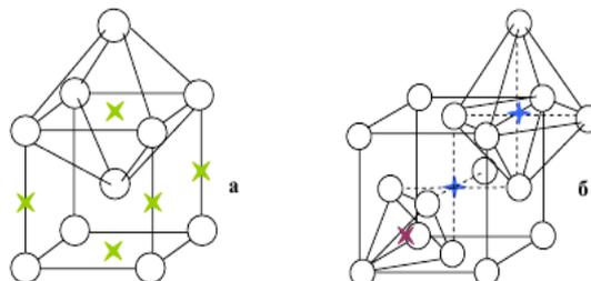
Picture 1. Possible locations of solute atoms (marked with asterisks) in the interstices of metal crystal lattices: body-centered cubic (a) and face-centered cubic (b)
