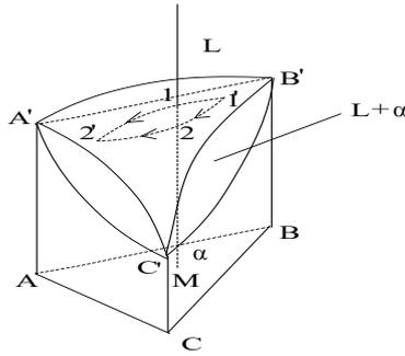
Thus, knowing the properties of an equilateral triangle, the position of the figurative point can be used to estimate the composition of the three-component alloy, or, knowing its composition, the position of the figurative point in the plane of the concentration triangle can be found.
