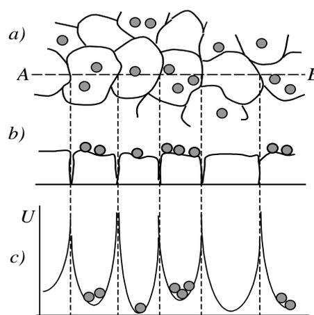
Fig.25. 4 . Distribution of catalyst atoms over regions of free migration of the catalyst: geometric barriers on the support surface ( a,b ); energy barriers on the surface of the carrier ( c )
