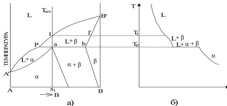
Rice. 6.6. Diagram of the state of a peritectic type system (a) and cooling curve of alloy  $x_1$  (b).
