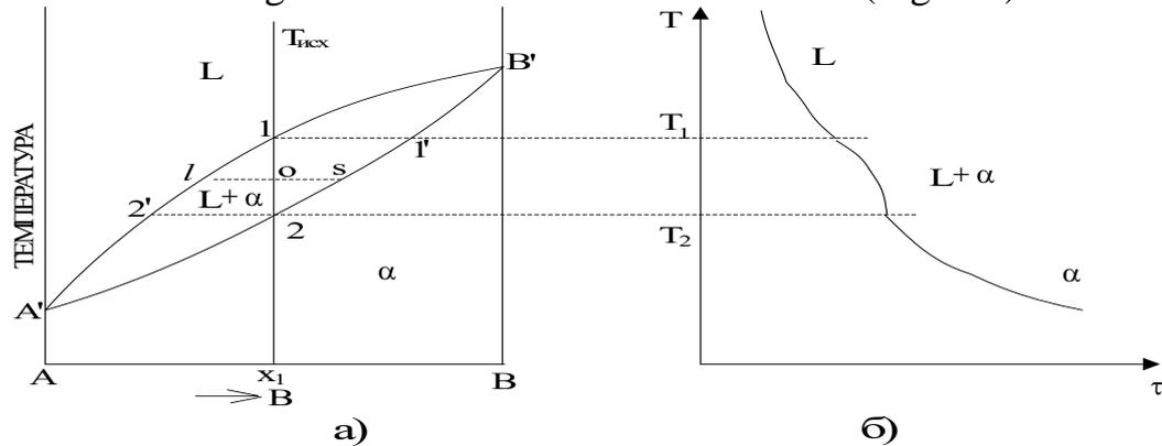
Рис. 6.4. State diagram of a system with unlimited solubility of components (with the formation of a continuous series of solid solutions) (a) and cooling curve of the alloy  $x_1$  (b).
