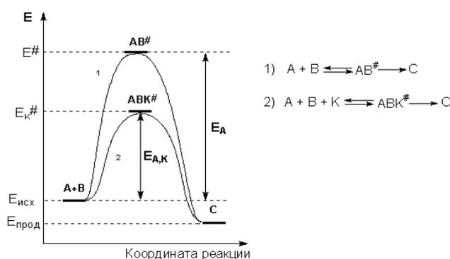
**Rice. 2.8** Energy diagram of a chemical reaction without a catalyst (1) and in the presence of a catalyst (2).
