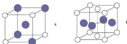
Figure-2. unit cells of crystal structures of substitutional solid solutions: a – disordered solution based on a body-centered cubic structure; b – ordered substitution solution based on a face-centered structure .
