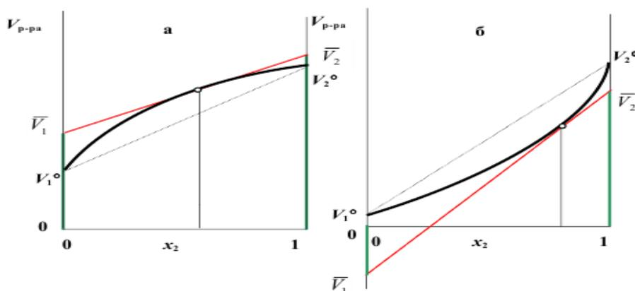
Figure 13 – Determination of partial molar volumes of components of a binary solution by a graphical method for solutions with decompression (a) and solutions exhibiting compression (b)
