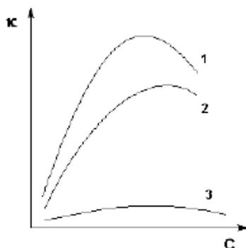
Rice. 20. Dependence of the specific electrical conductivity of electrolytes on concentration: 1 – H<sub>2</sub>SO<sub>4</sub>; 2 – KOH; 3 – CH<sub>3</sub>COOH.
