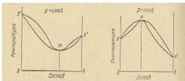
According to Konovalov's II law, at points C the composition of the vapor coincides with the composition of the liquid. Unlike all mixtures, azeotropic mixtures (corresponding to point M) will turn into vapor without change when the pressure decreases.
