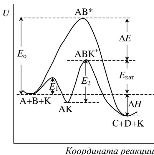
Rice. 24.1. Non-catalytic and catalytic reaction pathway profiles .
