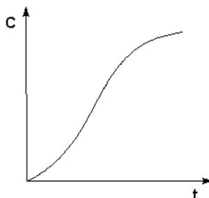
Rice. 2.9 Kinetic curve of the product of an autocatalytic reaction
