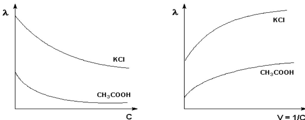
**Fig.3.** Dependence of molar electrical conductivity on concentration. **Fig.4.** Dependence of molar electrical conductivity from dilution
