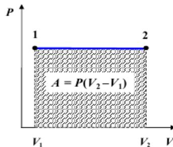
Figure 3 – Work of gas expansion in an isobaric process
