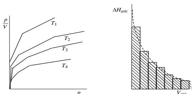
Rice. 25.1. Gas adsorption isotherms Fig. 25.2. Heat of gas adsorption on a solid adsorbent at different conditions on the catalyst surface temperatures: ( $T_1 > T_2 > T_3 > T_4$ )
