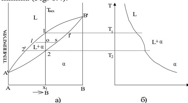
Rice. 6.4. State diagram of a system with unlimited solubility of components (with the formation of a continuous series of solid solutions) (a) and cooling curve of alloy x1 (b).
