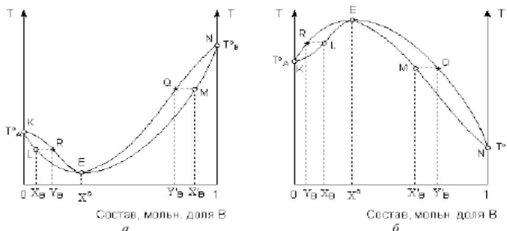
*Rice. 14. State diagrams of solution - vapor for volatile solutions of the 2nd type in the coordinates boiling point - composition for systems with a minimum (a) and maximum (b) boiling point*
