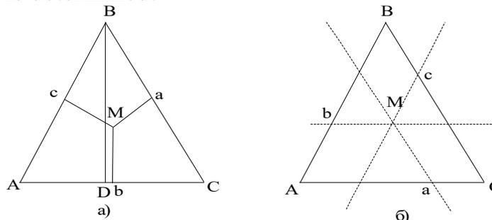
Rice. 6.9. Properties of an equilateral triangle applied for depicting the compositions of three-component alloys.
