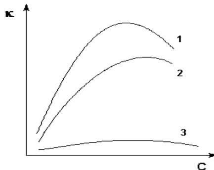
**Rice. 2.** Dependence of the specific electrical conductivity of electrolytes on concentration (1 –  $\text{H}_2\text{SO}_4$ , 2 –  $\text{KOH}$ , 3 –  $\text{CH}_3\text{COOH}$ ) .
